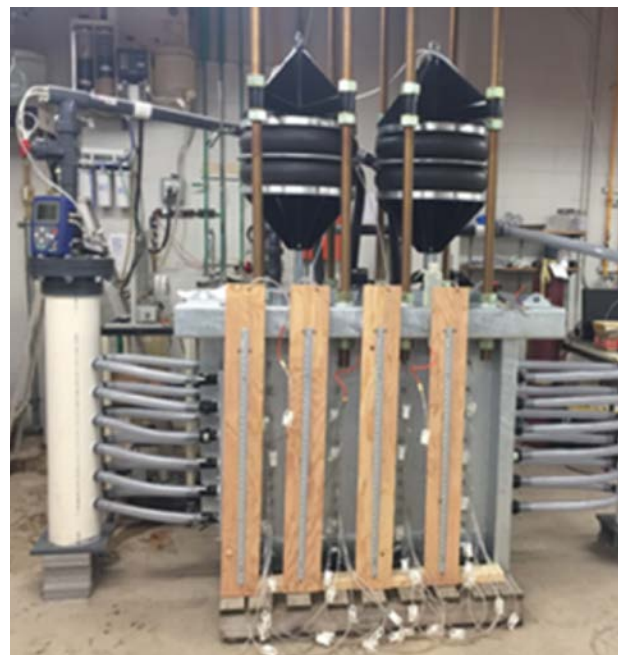
Purpose-built 2-D permeameter
